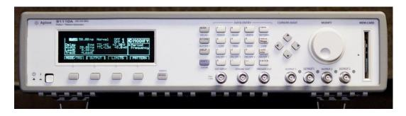
The 81110A pulse generators in Computer Hardware Design lab have a single channel 81112A module installed. The output channel is capable of 3.8V/ 330 MHz max. The pulse generator saves your setting prior to power down. For ease of use, a good starting (CHD lab1) point is stored (1). After powering up the Pulse Generator, **recall 1** should provide the following settings:
