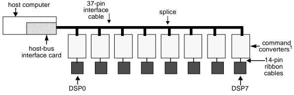
Notes: 1. There is a jumper setting on each command converter to select address, DSP0...DSP7.
