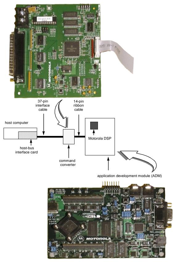
Figure 1-8. Parts of the Hardware Debugger (ADS)
