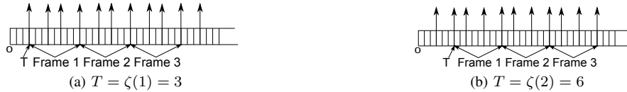
Fig. 2. Partition of time-line into frames when \lambda_p = \frac{3}{8} . Each small rectangle represents a time-slot. The arrival of a primary packet at the transmission queue of PT during any slot is indicated by a vertical arrow at the boundary between the slot and the one immediately after it.
