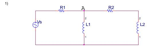
a). In the above circuit, find a differential equation for the current through L2, IL2(t). The source is an arbitrary source. (Hint: Consider applying KCL at A and determine an expression for VA in terms of IL2.)
