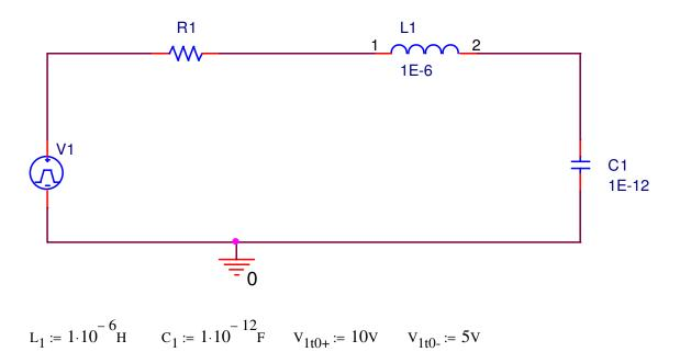
In the circuit above, the voltage source is 5V for t<0 and 10 V for t >0.
