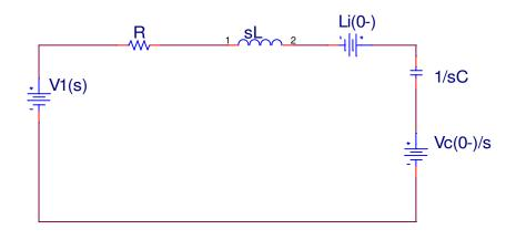
$I_L(0-) = I_L(0+) = 0$  DC steady state for components so capacitor is open so the current in series circuit in 0.
