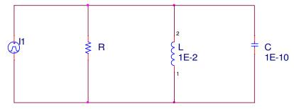
In the above circuit, the source current is 20mA for t < 0 and 0 for t > 0 (the source turns off at t = 0).
