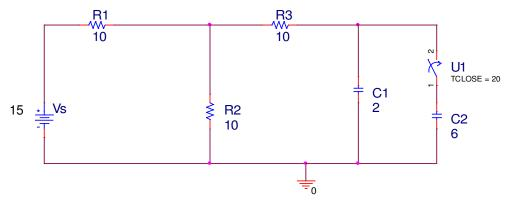
In the above circuit, the source turns on at t = 0 with a voltage of 15V, Vs=15u(t)V. Additionally, at t = 20s the switch in series with C2 is <u>closed</u>. You can (should) ignore C2 for part a) of this problem.
