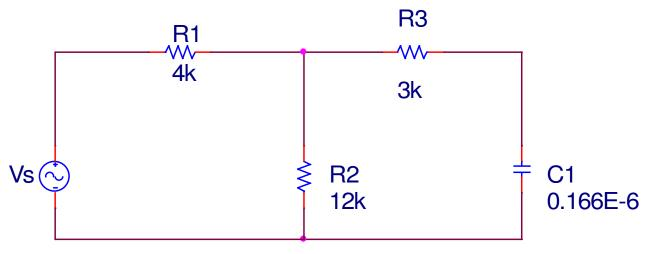
The source is a 5V sinusoidal signal with a frequency of 239.7Hz and has a zero phase.
