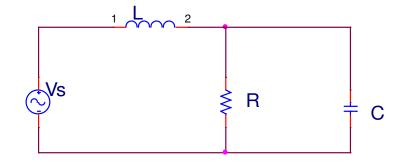
Determine the transfer functions in the following circuit. Determine the behavior of the transfer function as  $\omega$  goes to 0 and  $\omega$  goes to  $\infty$ .
