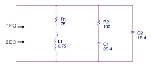
a. Determine the equivalent admittance,  $Y_{EQ}$ , for the above circuit for a frequency of 15.9 Hz. Determine the equivalent impedance,  $Z_{EQ}$ .
