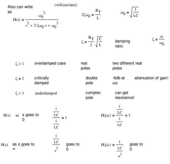
This is a low pass filter and a rolloff of 40db pole  $\omega^2$  or  $s^2 = 2 \times 20 \log 100$ ()
