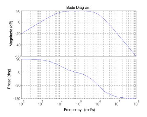
b. Determine the transfer function for the following magnitude and phase Bode plots (the plots are for the same circuit).
