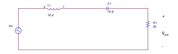
a. Determine the transfer function for the above circuit,
