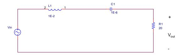
a. Determine the transfer function for the above circuit  $H(s) = \frac{V_R(s)}{V_{in}(s)}$
