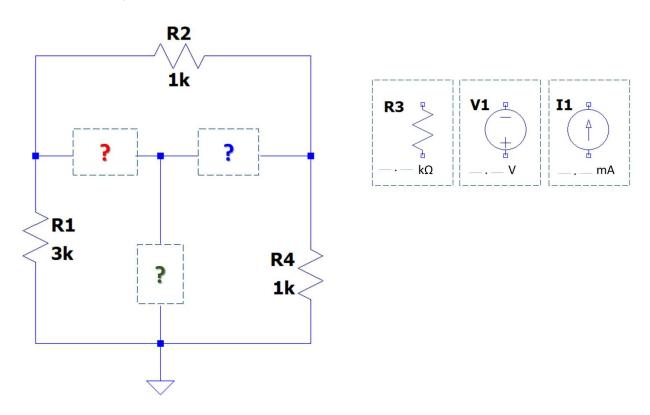
1.1: (1 pt) Step 1: Redraw your circuit below. *Include your reference marks across the resistor for your passive sign convention "scaffolding"*. Ground must be where it is originally placed. You can turn your components and give them any polairty you'd like. (Note: Reference marks are absolutely necessary to draw on your circuit. Without them, your 1.2 step will be marked incorrect with no partial credit!)
