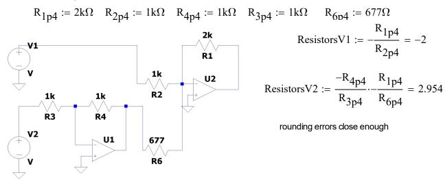
inverting summer but V2 must have a inverting amp before it. need correct ratio of resistors 2 in first op amp, 3 is second. Don't have to draw power sources in for this one.
