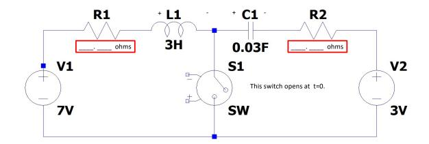
In the above circuit, switch S1 is closed (shorted) for t<0 and opens at t=0. Be careful with polarities which are indicated for L and C. Write your values for R1 and R2 using integers (1-9). Do not use 0.
