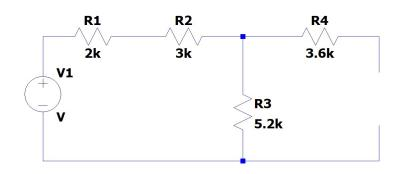
$$V_{11c1} \coloneqq 7V \qquad R_{11c1} \coloneqq 2000\Omega \qquad R_{21c1} \coloneqq 3000\Omega \qquad R_{31c1} \coloneqq 5200\Omega \qquad R_{41c1} \coloneqq 3600\Omega$$
