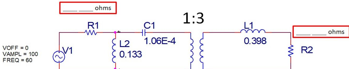
2.1: **30 pts**) Choose the values of R1 and R2. (i.e 15 ohms and 78 ohms. respectively...) **You may use either referral method though one referral method is one less step. (30 pts)**
