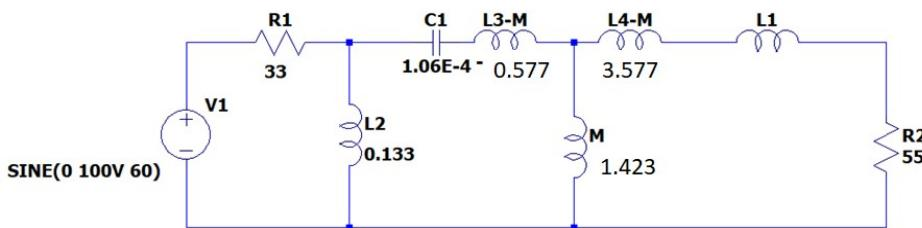
To find VR2...can use circuit reduction and then voltage divider...make equal to find L1
