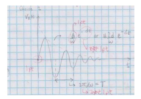
2.4: Analytically calculate the circuit components that represent of the pole zero diagram. Show that these circuit components result in the time domain plot you calculated/estimated using methods <u>from Differential Equations</u>. The source is a step function and you may choose the value of your step function source.
