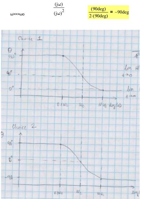
ω << ω o  $\frac{(jω)}{2.9 \cdot 10^7}$ (90deg) = 90deg  $\frac{(jω)}{(jω)^2}$   $\frac{(90deg)}{2 \cdot (90deg)} = -90deg$
