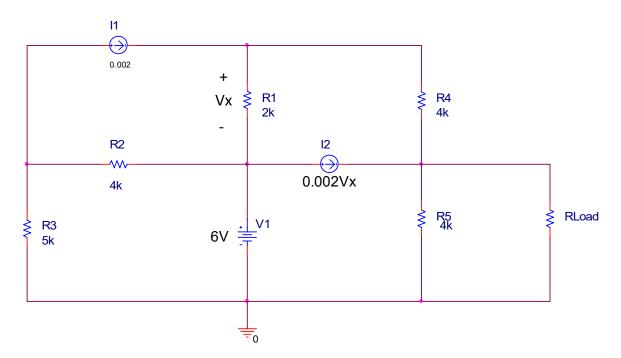
a) Determine VTH using any analysis method, IN using any analysis method, and RTH using the test method for the above circuit. Verify your answers.
