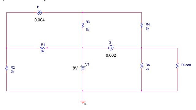
On the above circuit, using any method, find the a) thevenin voltage, b) thevenin resistance, and c) norton current. Draw the schematics of the norton and thevenin circuits for full credit. Confirm your values by any method.
