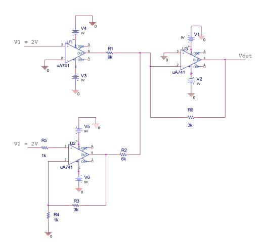
a) Find the output voltage, Vout. The voltages to power the op-amps are 9V and -9V.
