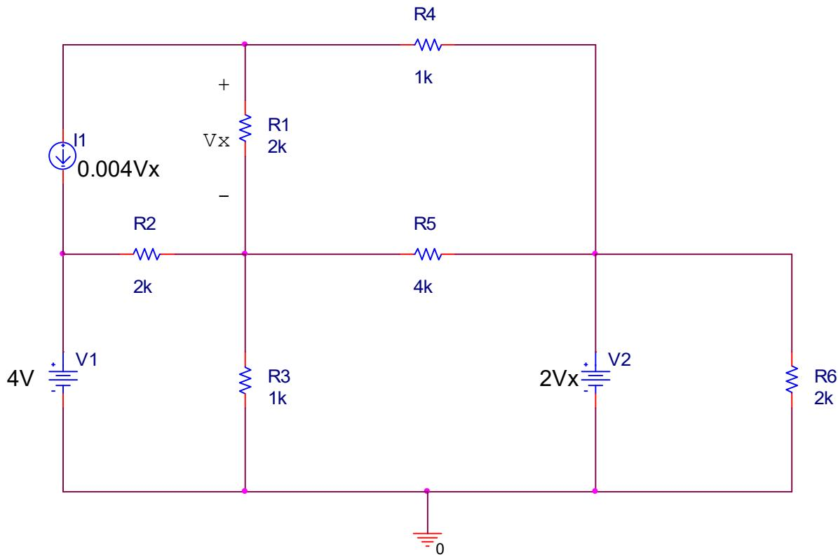
In the circuit above, set up the linear system to analyze the circuit using both mesh and node analysis. You only need to solve for  $V_x$  using one of the methods. Be sure to include the following:
