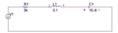
At  $t = 0^{-}$ , the voltage across the capacitor is 5V (polarity shown), the current through the inductor is 2mA to the 'right' and the source is 10V. At  $t = 0^{+}$ , the voltage source becomes 5V and doesn't change for t > 0.
