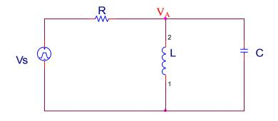
a. In the above the circuit, find the differential equation for the voltage across the capacitor C, VC(t). The source is an arbitrary source.
