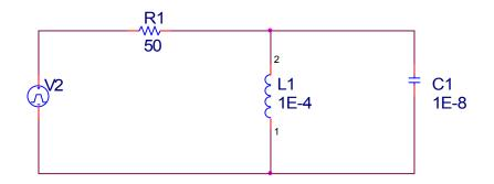
At  $t = 0^{-}$ , the voltage across the capacitor is 8V, the current through the inductor is 10mA 'downward' and the source is 10V. At  $t = 0^{+}$ , the voltage source becomes 3V and doesn't change for t > 0.
