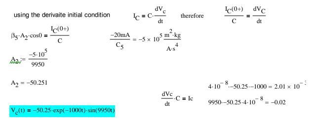
Now we must use the differential relationship IC=dVc/dt to obtain the current through the capacitor  $I_c(t) = 2.01 \cdot 10^{-3} \cdot \exp(-1000t) \cdot \sin(9950t) - 0.02 \cdot \exp(-1000t) \cdot \cos(9950t)$
