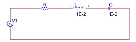
In the above circuit, the source voltage is 5V for t<0 and 10 V for t>0
