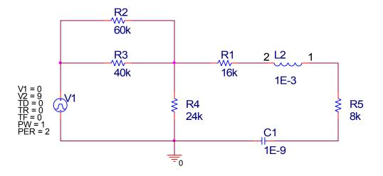
In the above circuit, the initial conditions are zero and the source can be considered a step function, 9u(t).
