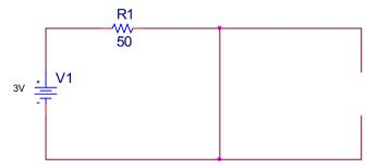
At steady state, the inductor is a short and the capacitor is an open circuit
