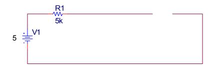
At steady state, the inductor is a short and the capacitor is an open circuit
