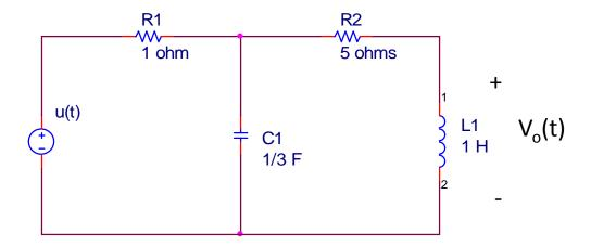
2.1: Draw the s-domain equivalent circuit. Assume all intial conditions are zero and the source is an arbitrary source.
