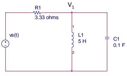
$v_S(t) = 10 \, u(t)$  AND assume that -1A flows through the inductor and +5V is across the capacitor at t=0....i.e. vc(0)=5 and iL(0)= -1
