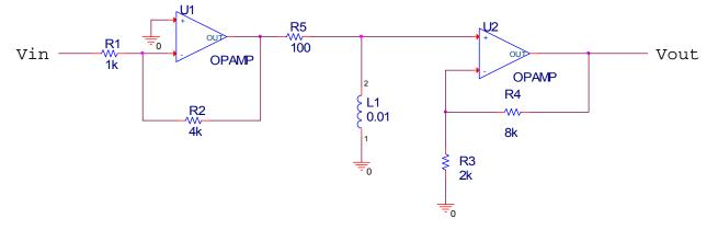
2.1 Draw the above circuit as a three stage network (put boxes around the stages for example and label Hn(2) n=1,2.3...etc). Indicate the tranfer function for each stage.
