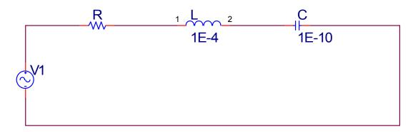
3.1. What is the resonant frequency of the circuit?
