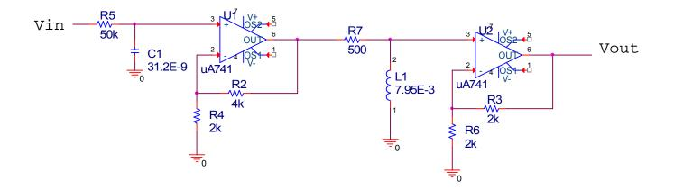
2.8. Draw the above circuit as a three stage network (put boxes around the stages for example and label Hn(2) n=1,2.3...etc). Indicate the tranfer function for each stage.
