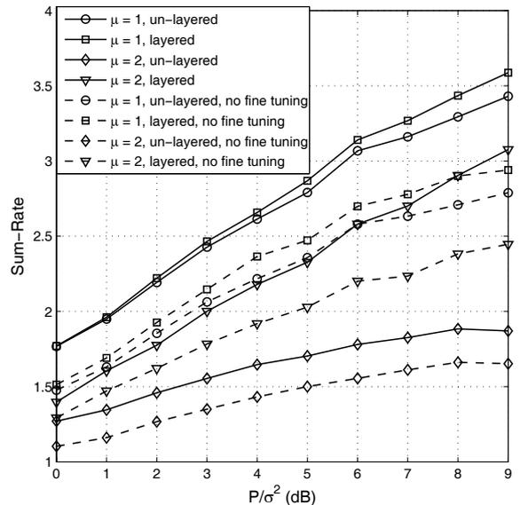
Fig. 7. The optimal predicted sum-rate under practical modulation and coding schemes.
