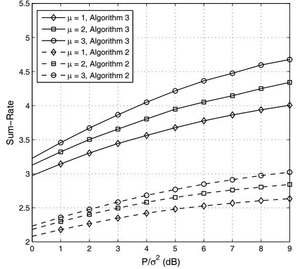
Fig. 2. The sum-rate given by Algorithms 2 and 3 assuming Gaussian signaling and infinite-length random codes.
