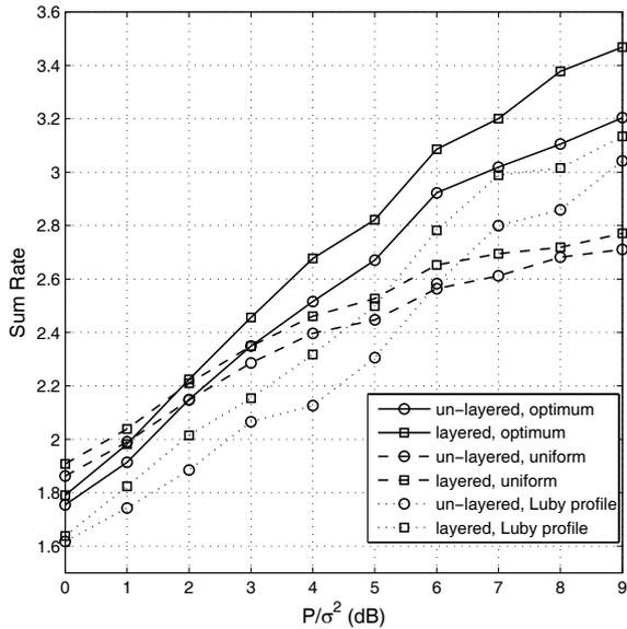
Fig. 9. The simulated throughput with QAM and optimized rateless codes.
