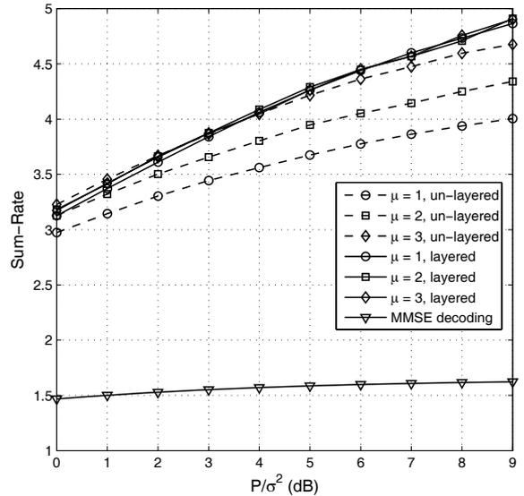
Fig. 4. The sum-rate given by Algorithm 3 assuming Gaussian signaling and infinite-length random codes.
