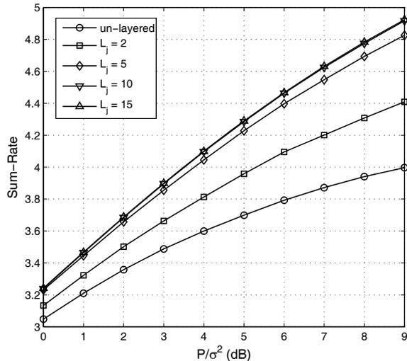
Fig. 3. The sum-rate given by Algorithm 3 assuming Gaussian signaling and infinite-length random codes for different number of layers.
