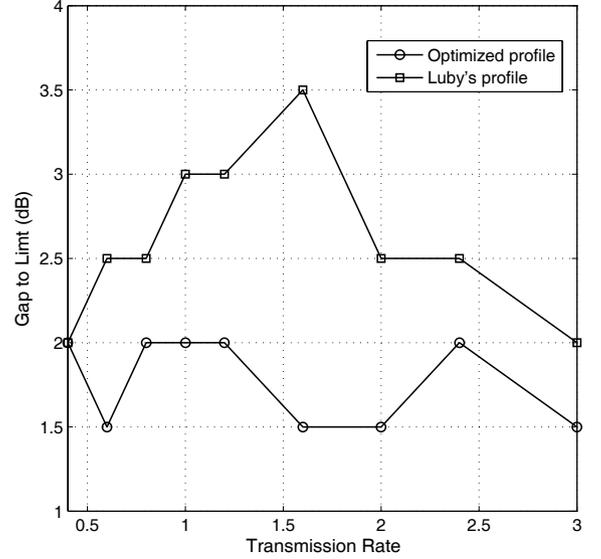
Fig. 8. The gap to Shannon limit for the optimized profile and Luby's profile.
