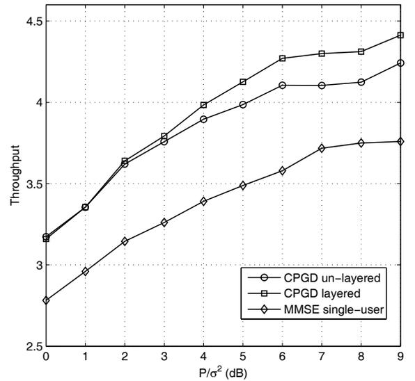
Fig. 10. The simulated throughput in MISO channel with beamforming.
