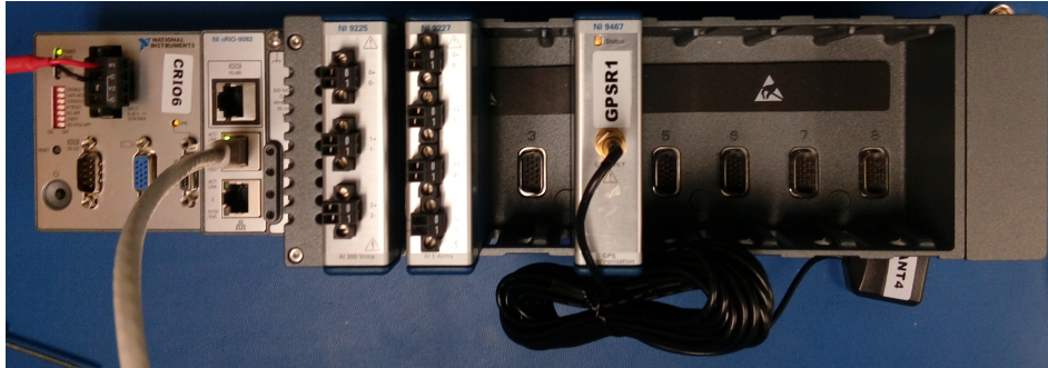
Figure 2.3: Physical PMU Hardware in a Compact-RIO 9068
