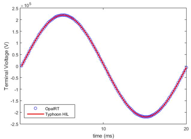
Fig. 5: Response of the transformer model while subjected to rated input voltage
