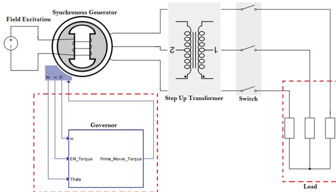
Fig. 2: Schematic of the Micro-system Developed in the Typhoon HIL Schematic environment (Red boxes represent the Governor model and the load model implemented as in Section III.A)
