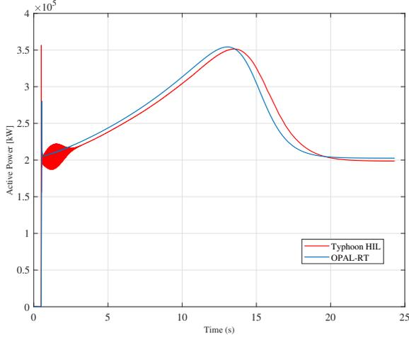
Fig. 6: Transient Response of the Motor
