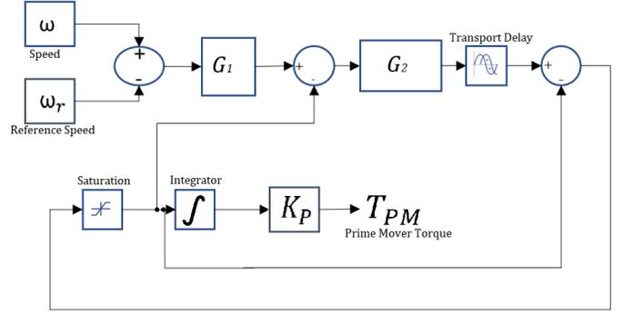
Fig. 1: Simplified Governor Model implemented using Typhoon HIL Schematic Editor
