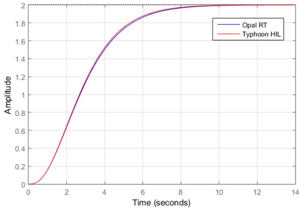
Fig. 4: Step response of the modeled governor
