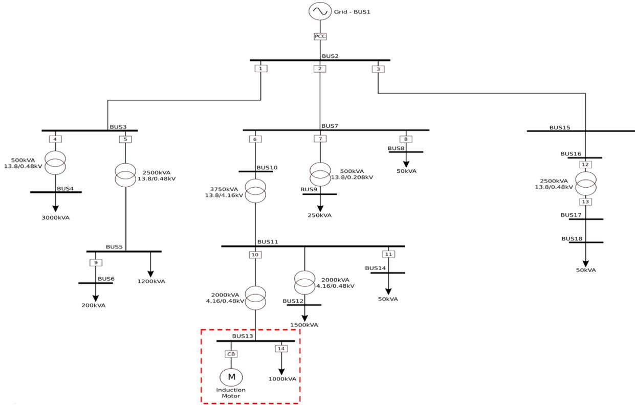
Fig. 3: Schematic of the Microgrid Developed in Typhoon HIL Schematic environment (the red box outlines the induction motor model described in Section III.A)
