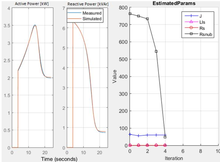
Fig. 7: PET parameter estimation results for  $J$ =Motor Inertia,  $L_{ls}$ =Stator Inductance,  $R_s$ =Stator Resistance,  $R_{snub}$ =Snubber Resistance
