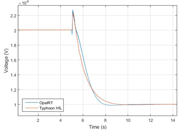
Fig. 8: Transient responses of the generator in the Micro-System
